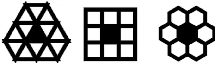
Hexagonal cells can be used to generate a uniform highly symmetric grid. Each cell shares both vertices and cell walls with its 6 neighbours. Square cells, with 8 neighbours and 4 wall neighbours and triangular cells with 12 neighbours and 3 wall neighbours have lower degrees of symmetry.
