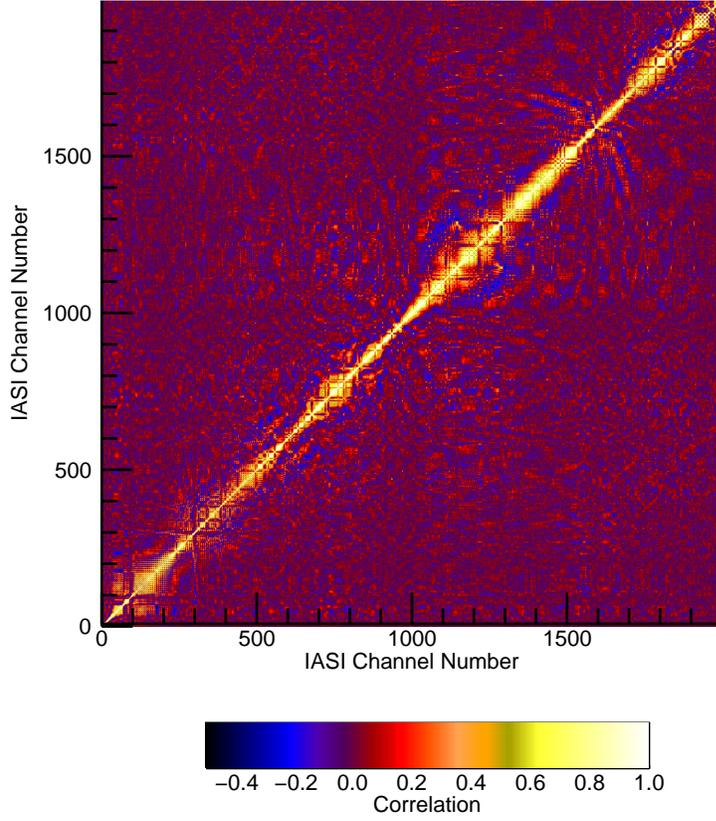
Fig. 2: The noise error correlation matrix for IASI reconstructed radiances. Band 1 (645-944cm<sup>-1</sup>) only.
