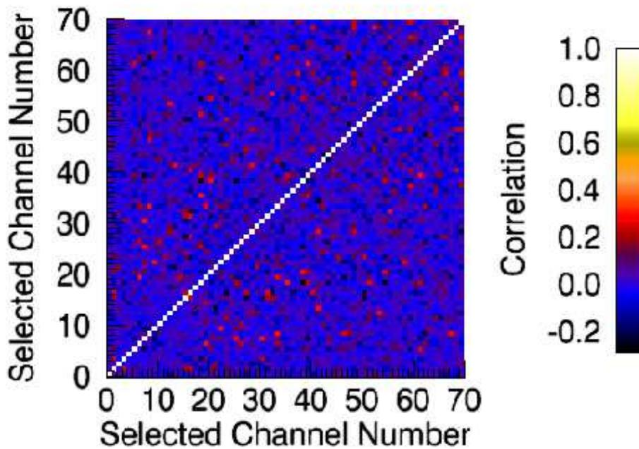
Fig. 8: The observation error correlation matrix for the 70 channels chosen in the reconstructed radiances channel selection when the inter-channel correlation is limited to 0.3.
