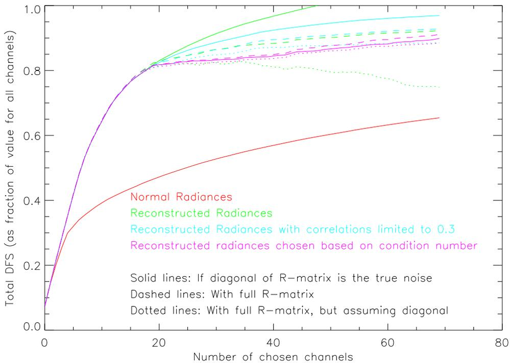
Fig. 12: As Figure 5 but the evolution of the degrees of freedom for signal for the condition number selection has been added. Although, perhaps unsurprisingly, the performance based simply on the condition number is poorer, its sensitivity to the three observation error assumptions is seen to be low.
