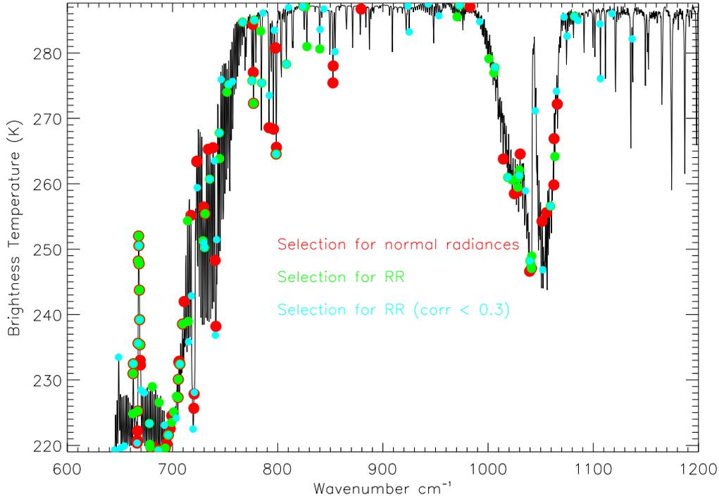
*Fig. 6: A typical IASI spectrum upon which are plotted the selected channels for the three scenarios considered here. The red dots are for the normal channel selection, green is for reconstructed radiances and cyan is where the absolute inter-channel correlation is limited to be less than 0.3.*
