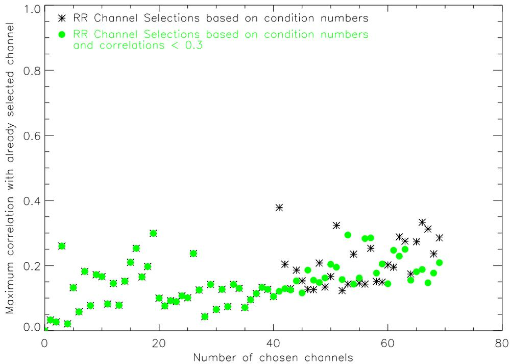
Fig. 11: Maximum correlation for each new channel for the condition-number based channel selection.
