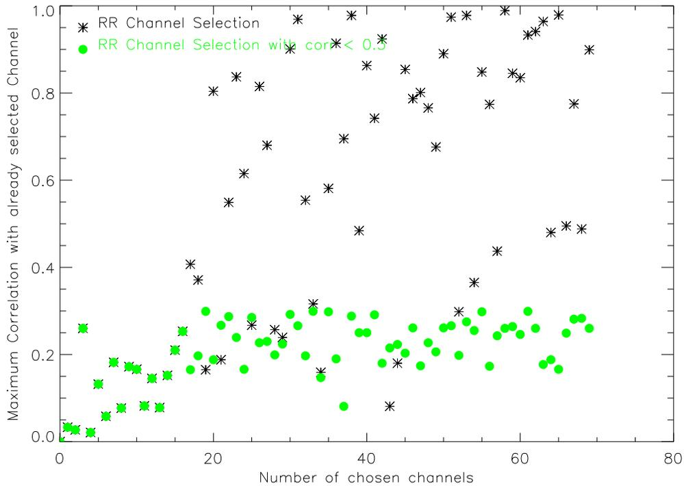
*Fig. 4: The evolution of the maximum inter-channel error correlation for the reconstructed radiances channel selection with and without the imposition of a maximum value of 0.3.*
