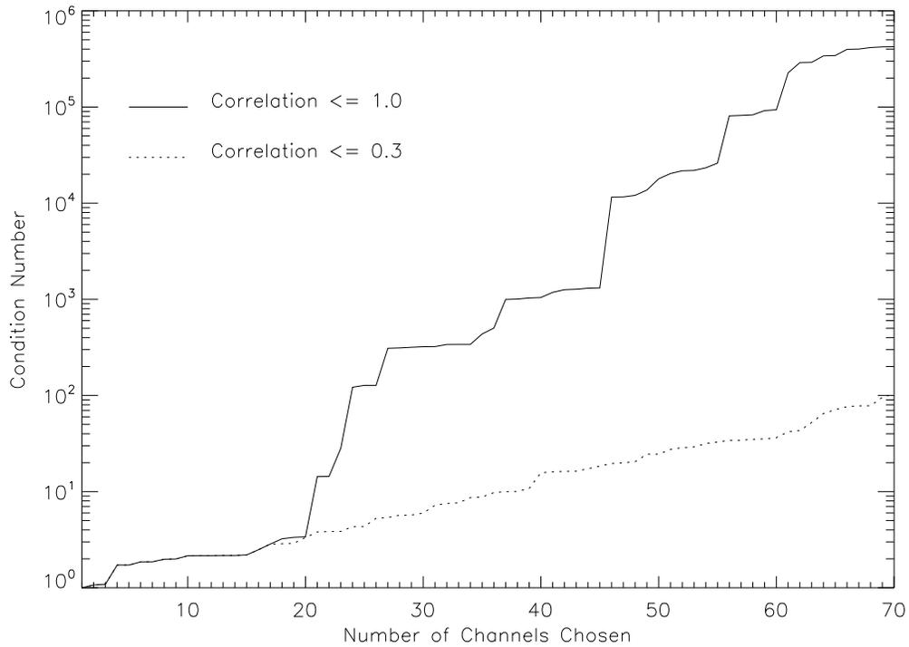
Fig. 9: The condition numbers of the observation error covariance matrix for the reconstructed radiance channel selections in Figure 5. The selection where correlations are limited to less than 0.3 are far better conditioned.
