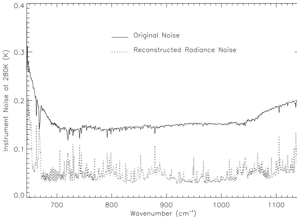
*Fig. 1: The diagonal of the level 1c IASI instrument noise error covariance matrix for original and reconstructed radiances. Band 1 (645–944 cm<sup>-1</sup>) only.*
