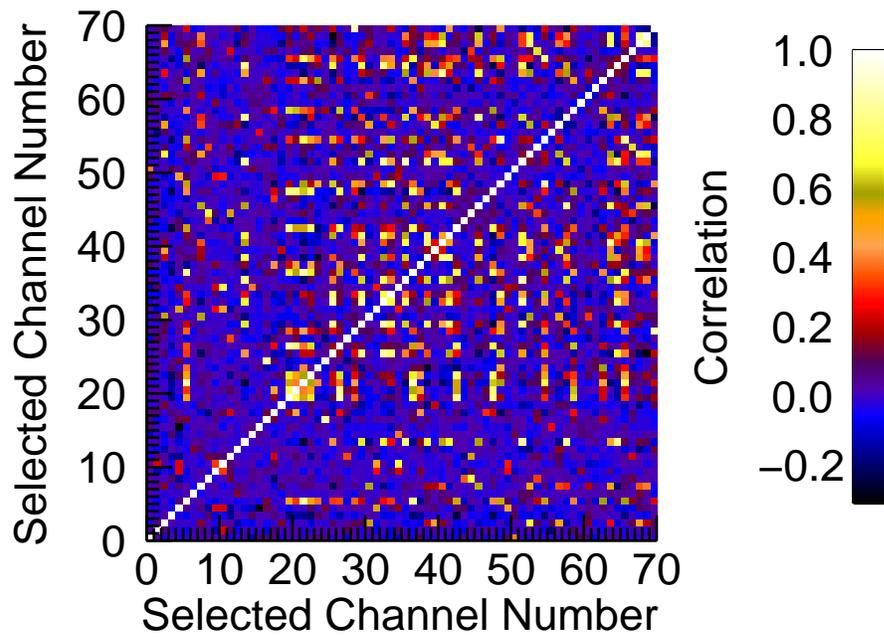
Fig. 7: The observation error correlation matrix for the 70 channels chosen in the reconstructed radiances channel selection. The channels are in the order in which they were chosen.
