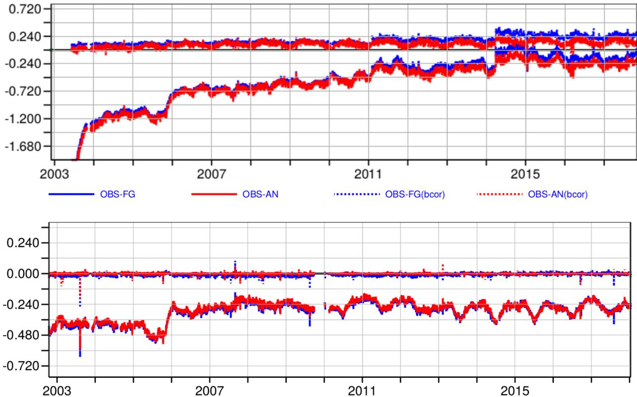
The lower panel shows the same time series for AIRS 787 in ERA-5 where the bias initialisation problem was addressed. There is now no evidence of a drift in this channels and it is believed that this is a much more realistic representation of the excellent stability of this channel and the AIRS instrument in general.
