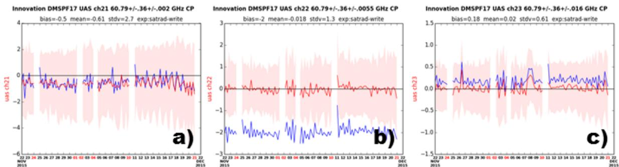
**Figure 5.** A time series of the global bias and standard deviation for SSMIS channels 21 (a), 22 (b) and 23 (c). The global mean departure without bias correction is shown in blue, after bias correction in red, and the standard deviation is for the bias correct departure is shown in red shading.
